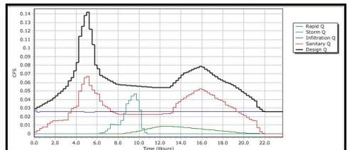
Four types of hydrographs: Sanitary, Storm, Groundwater, Rapid Infiltration
