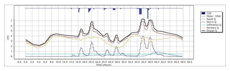
There is a new feature to make it easier to compare results hydrographs between different entities or analysis scenarios. A new "Design Q to Flow Meter" button in the Hydrograph tab automatically creates a Flow Meter data set for the total hydrograph (Design Q). All you have to do is type in a name for it, and then select it in the FLOWMETER field in the collection system layer Properties grid. Then the dark red "Meter" hydrograph will display for that entity.
