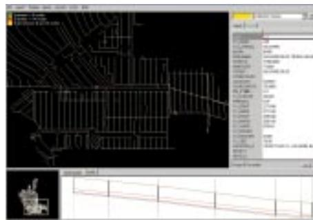
**A visual query of pipe diameters in Pizer's Hydra™ Hydraulic Modeling Software, used in the city of Beverly Hills Sanitary Sewer Collection System Master Plan.**
